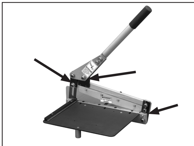
Figure 6. Lubrication locations (left side shown).
